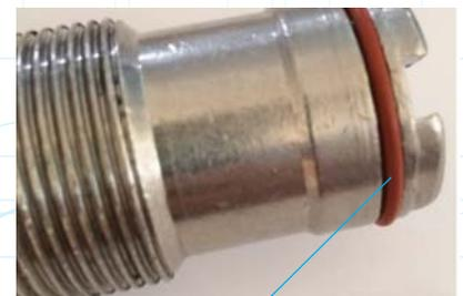
*Particular attention needs to be paid to sealing areas ensuring that no damage is present that can compromise the integrity of the O-rings. Delavan strongly recommends the replacement of these O-rings each time the nozzle is assembled.*
