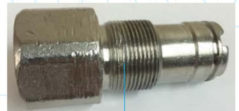
*Damage to threads on SDX III Nozzle*
